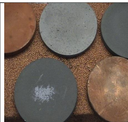
Figur 3. Metal-ceramic filter elements obtained by the method of CVD impregnation of porous structures.
